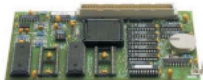
Panel control unit for installation in 8008 fire alarm panel.
