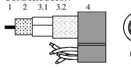
1 Inner conductor Solid soft annealed copper
