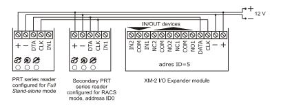
The maximum length of the cable run between a PRT reader and an XM-2 module and optional secondary PRT reader is limited to 150 m. For two-way door control the primary PRT unit needs to be configured for *Full Stand-alone* mode while the second (slave) reader needs to be configured for **RACS Online mode** with address set to **ID=0**.
