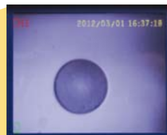
Image viewed through coaxial illumination below shows clean connector downloaded from SD card with time and date of image capture
