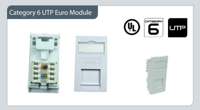
Category 6 Unshielded Twisted Pair (UTP) 25x50mm shuttered, moulded, modules (Euro Mod) conform to class E performance. They feature a slim line design, which is an ideal solution for shallow floor box or dado trunking applications.
