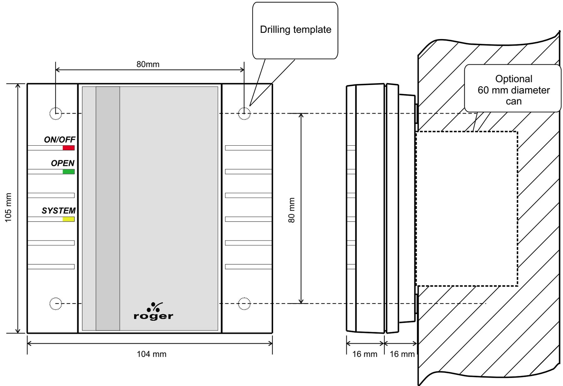
The front and side view of PR201 controller and PRT21 terminal.
