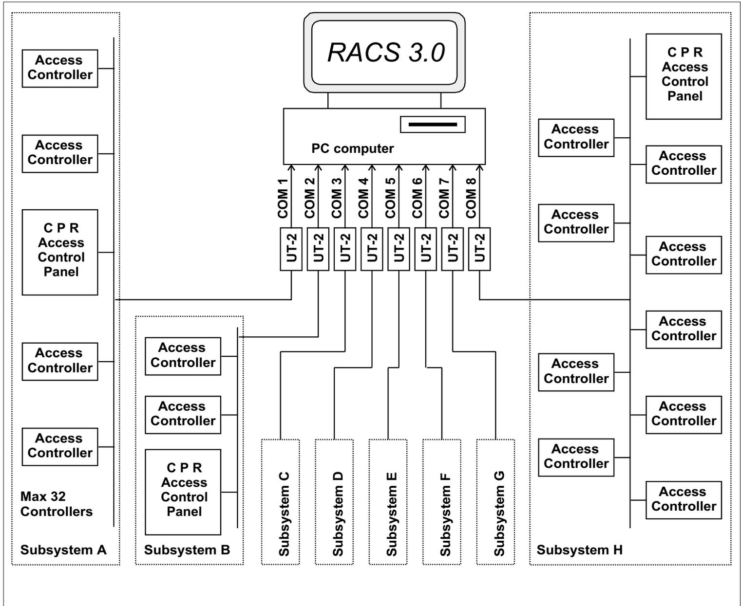
1. Every subsystem must be connected to separate COM port via UT-2 interface.
