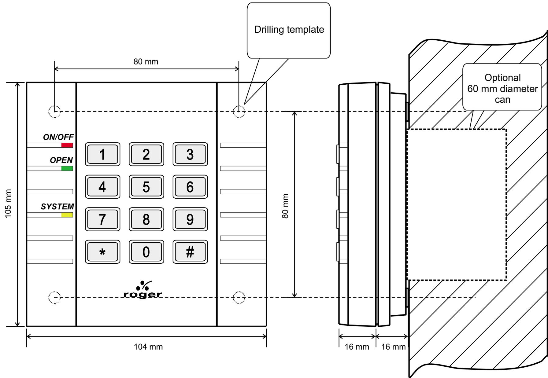
The front and side view of PR301 controller and PRT31 terminal.
