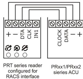
When operating with RACS format, reader stores all pressed keys in a buffer and does not transmit them, until the [#] key is pressed. Each entry of PIN code must be followed by pressing the [#] key, which is treated as the end of a PIN code. In RACS format when IN1 is triggered, the PRT32 will stop reading cards and PINs till the moment when IN1 will be released.
