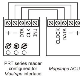
In *Magstripe* format, the PRT32 reader transmits a sequence of data bits representing either a code of the presented card or digits of entered PIN. When operating with *Magstripe* format, the reader stores all pressed keys in a buffer and does not transmit them until the [#] key is pressed — a press of the [#] key is treated as the end of the PIN code.
