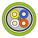
Type A for stationary applications (AWG 22/1 Solid Conductor)
