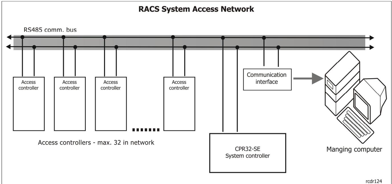
Generally, CPR32-SE works as centralized event buffer (250.000 events) and centralized clock for the entire access network. Also, it controls exchange of data between access controllers located within single access network which is necessary for so called "global functions" (e.g. APB Zones, Alarm Zones).
