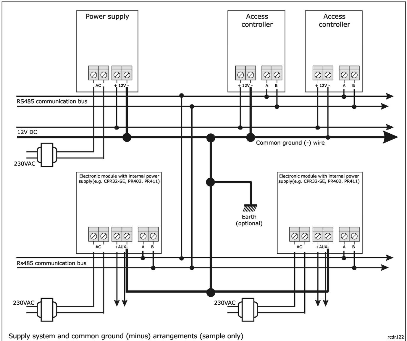
Note: It is forbidden to short positive (+) supply outputs from various devices working in the system.
