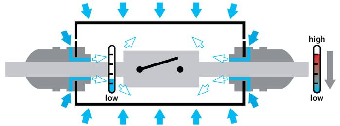
Through the usage of VentGLAND and VentPLUG, the interior pressure can adjust to the environmental pressure. The ingress protection class of the enclosure remains completely unchanged.
