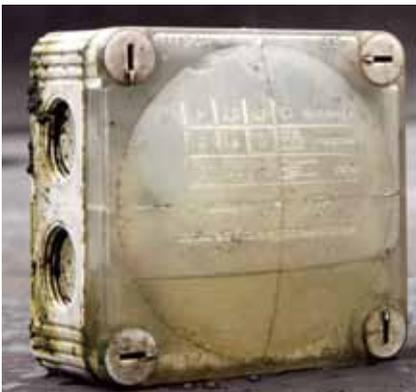
If the air in the enclosure cools down and there is no pressure equalization, condensation will form, which can no longer escape, as this example shows after two years of outdoor exposure.
